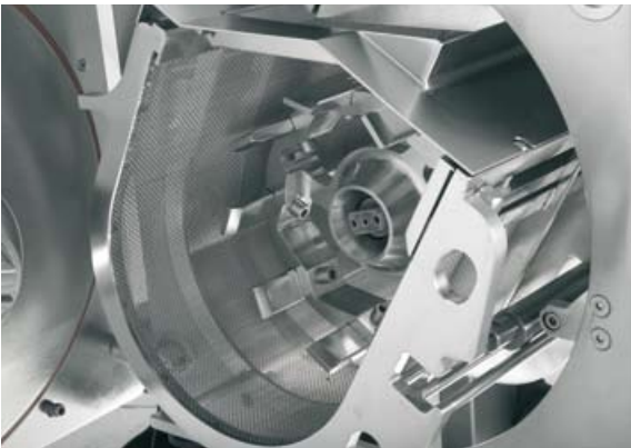
The final granulating step uses a fine rotor granulator from the RFG series (Picture shows the RFG 250 DDL, here shown with the pulled-out granulating mesh).
