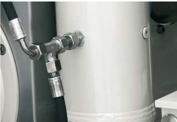
Control equipment and two hydraulic cylinders ensure the roller gap remains constant and with this the quality of the flake.
