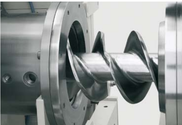
Alexanderwerk has decades of experience in the design of roller presses, which can be seen in the PP-Types: all modules of the PP 350 can be accessed easily. The picture shows the retraction of the feeding screw (without special tools).
