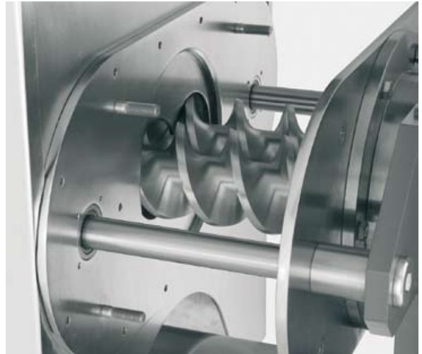
The design of the PP 250 reflects decades of experience in the construction of roller compactors: all modules are readily accessible. The picture shows how the feeding screws are swivelled and withdrawn (without any special tools).
