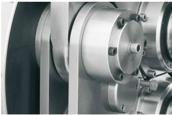
Control equipment and two hydraulic cylinders ensure the roller gap remains constant and with this the quality of the flake.
