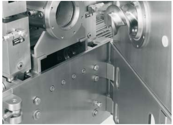
The compacting unit (left) and feeding unit (right) are connected to each other by hinges and are pivotable. They are screwed tightly together while the process runs.
