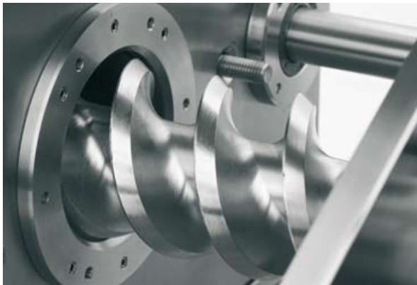
Alexanderwerk has decades of experience in the design of roller presses, which can be seen in the PP-Types: all modules of the PP 175 can be accessed easily. The picture shows the retraction of the feeding screw (without special tools).
